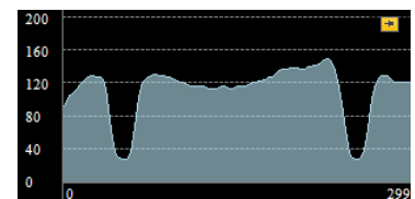
The image is scanned along the path and the brightness profile is extracted and smoothed.
