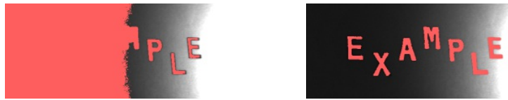
Results of ThresholdToRegion and ThresholdToRegion_Dynamic on images with uneven light.
