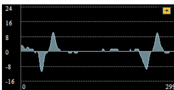
Brightness profile is differentiated. Notice four peaks of the profile derivative which correspond to four prominent image edges intersecting the scan line. Finally the peaks stronger than some selected value (here minimal strength is set to 5) are identified as edge points.
